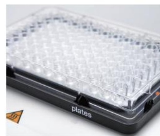
Temperature protection Block equipped with a lid for heat preservation
